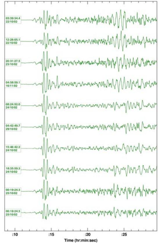
cluster analysis to group similar events together based on their cross-correlation coefficients at a given station. Master or reference events within each group are then used to determine consistent phase arrivals for all the events in each group. Then we used the double difference method of Waldhauser and Ellsworth (2000) to determine high-resolution hypocenter locations for the dataset. The results show improved clustering in the final hypocenters.
