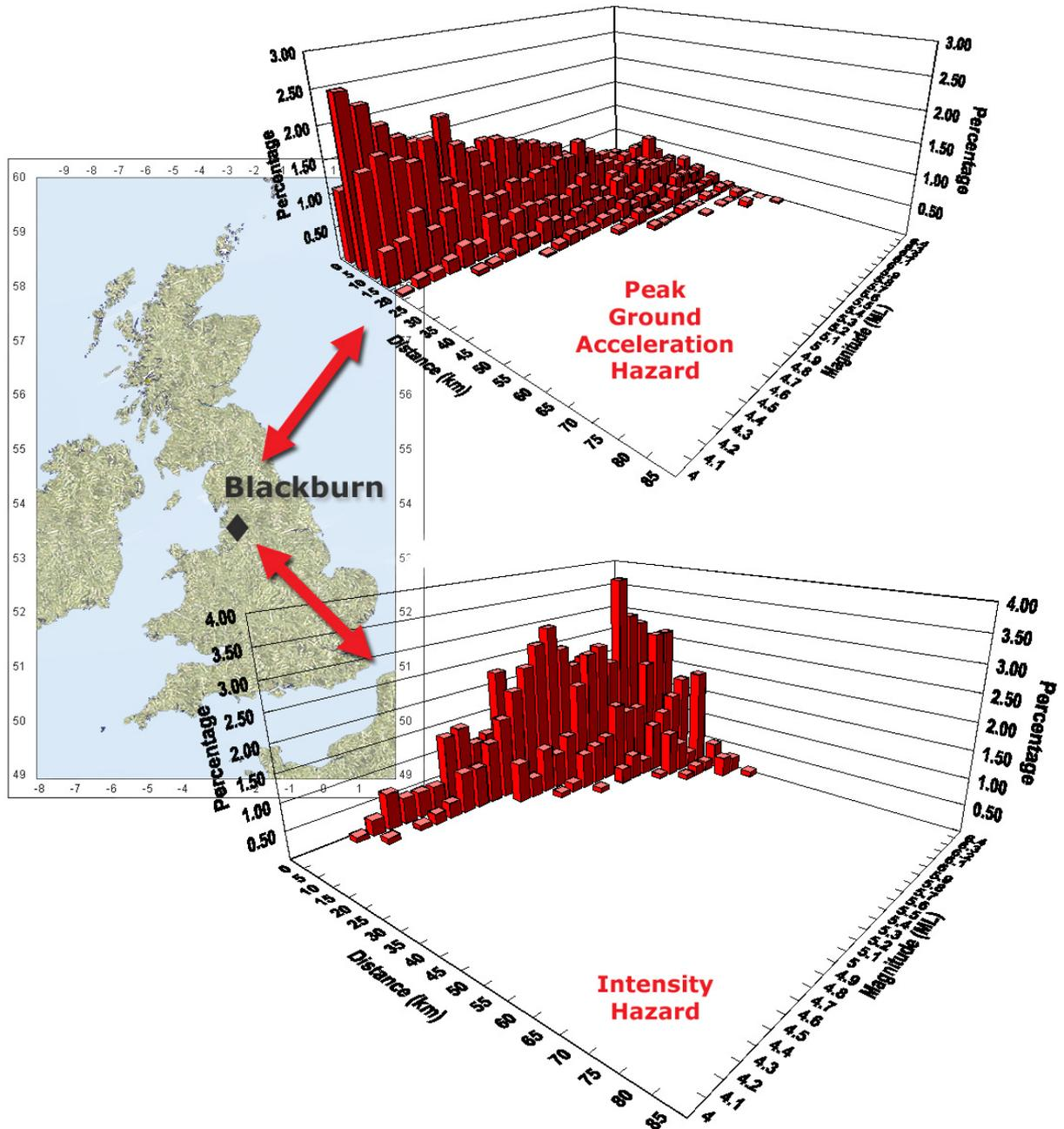
For an example site at Blackburn, frequency distributions are shown for different magnitude-distance combinations that would produce the PGA and intensity value that have an annual probability of occurring of 1 in 10,000. The two distributions are very unlike. Irregularities in the shape are due to the fact that the distributions were computed using simulations.
