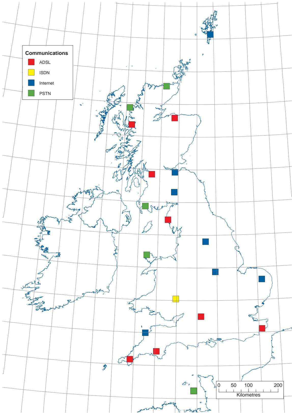
Communications links to UK seismograph network base stations.
