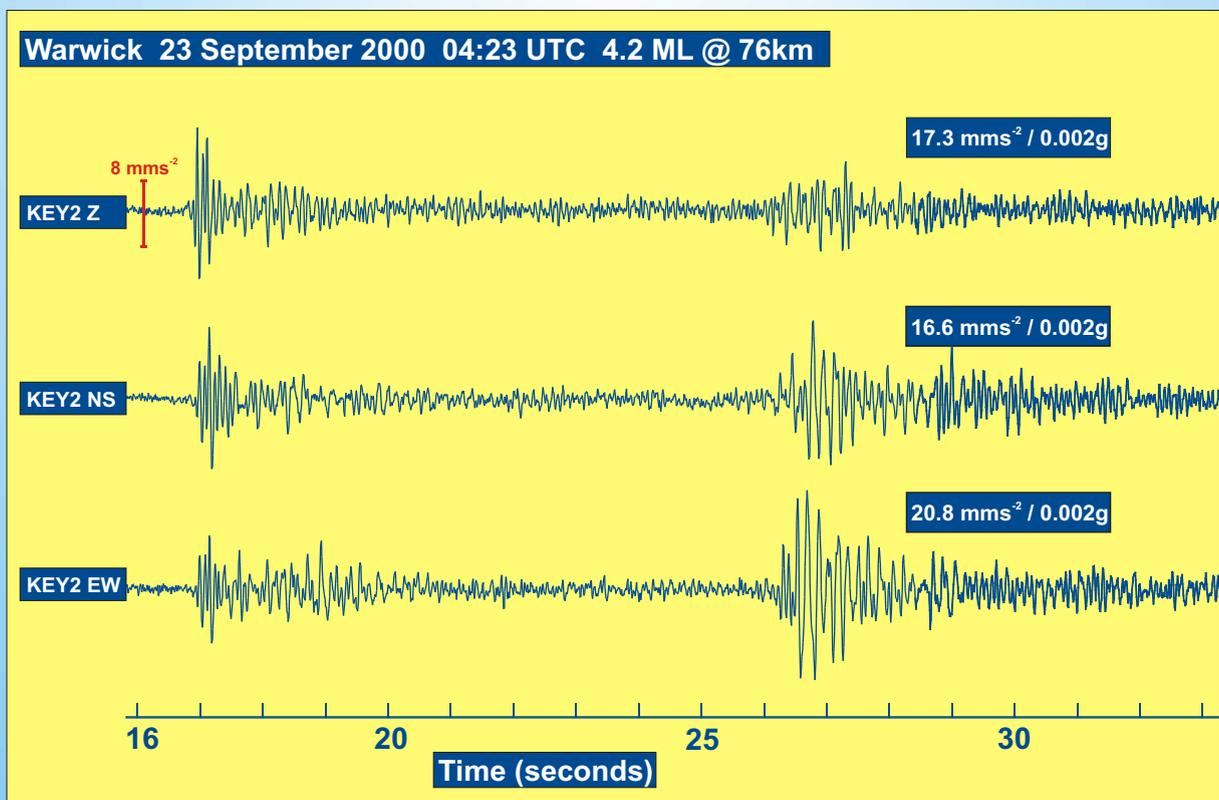
**Figure 16.** Seismograms recorded on the strong motion instruments near Keyworth from the Warwick earthquake with a magnitude of 4.2 ML on 23 September 2000 04:23 UTC. Three letter codes refer to stations in Annex E.
