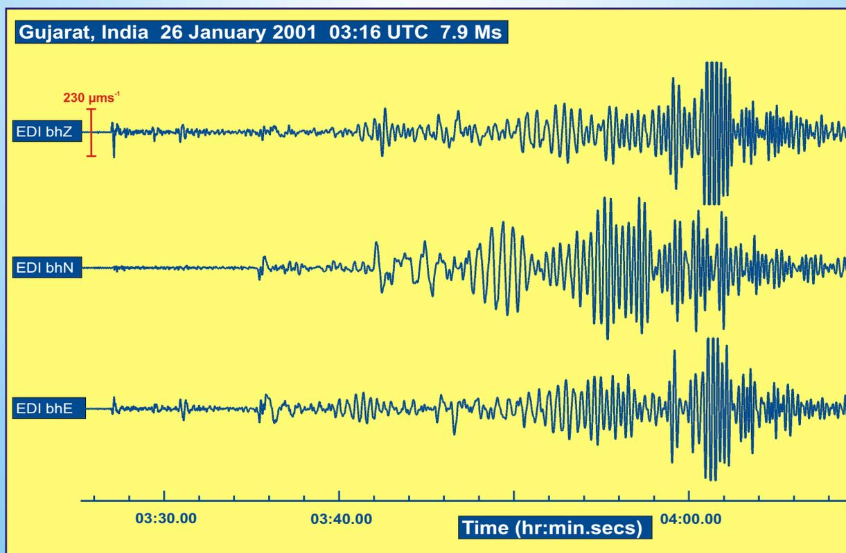
**Figure 22.** Seismograms recorded on the broadband instruments near Edinburgh from the Gujarat, India earthquake with a magnitude of 7.9 Ms on 26 January 2001 03:16 UTC. Three letter codes refer to stations in Annex E.
