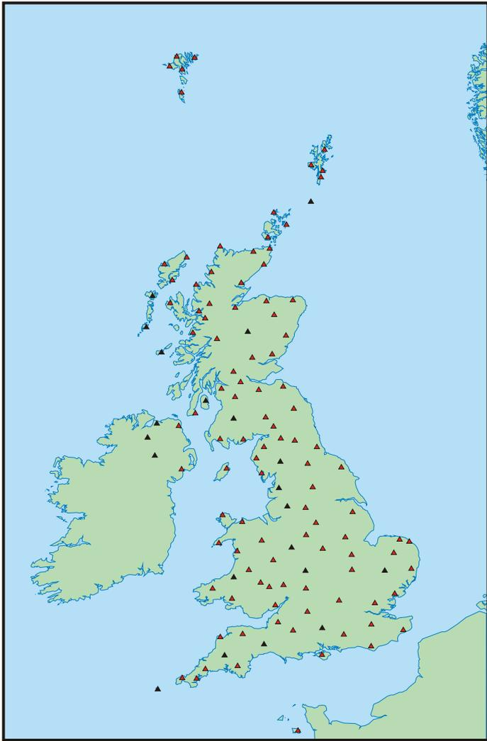
**Figure 5.** Proposed long-term background seismic monitoring network with an average station spacing of 70 km. Colour coding shows existing coverage (red) and proposed stations (black).
