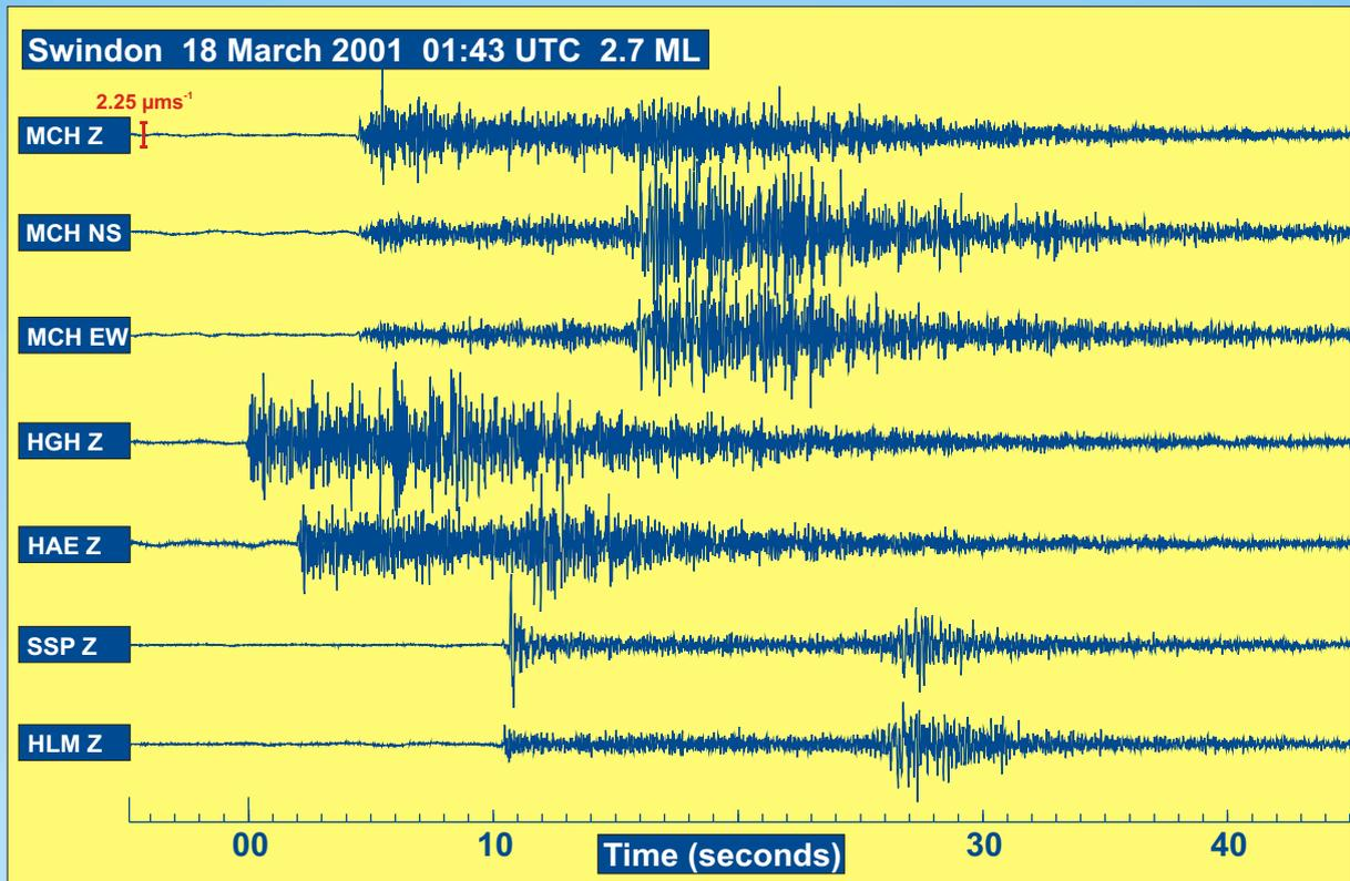
**Figure 17.** Seismograms recorded on the Hereford network from the magnitude 2.7 ML Swindon earthquake on 18 March 2001 01:43 UTC. Three letter codes refer to stations in Annex E.
