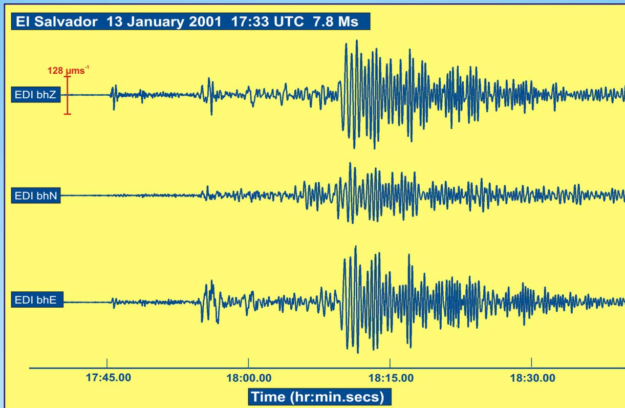
**Figure 21.** Seismograms recorded on the broadband instruments near Edinburgh from the El Salvador earthquake with a magnitude of 7.8 Ms on 13 January 2001 17:33 UTC. Three letter codes refer to stations in Annex E.
