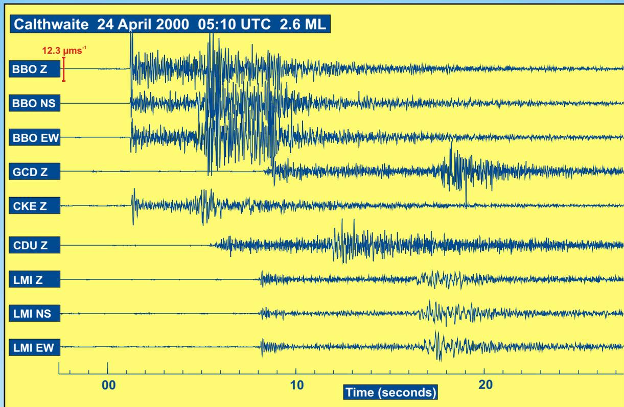
**Figure 13.** Seismograms recorded on the Cumbria network from the magnitude 2.6 ML earthquake felt in the Calthwaite area on 24 April 2000 05:10 UTC. Three letter codes refer to stations in Annex E.
