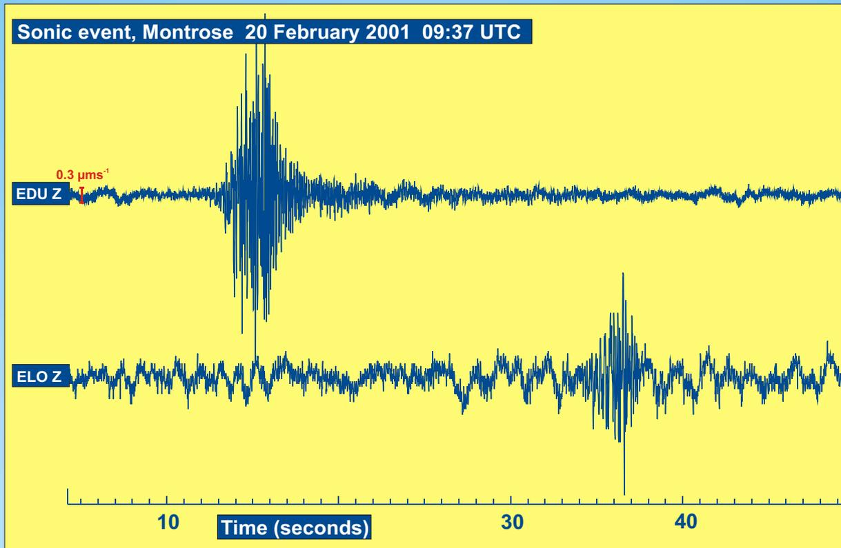
**Figure 19.** Seismograms recorded on the LOWNET (Edinburgh) network from the sonic event felt in the Montrose region on 20 February 2001 09:37 UTC. Three letter codes refer to stations in Annex E.
