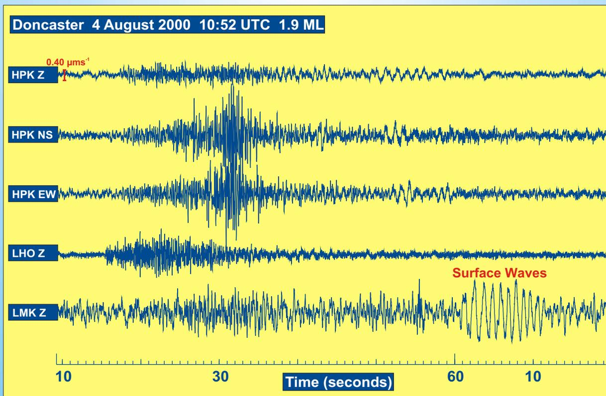
**Figure 18.** Seismograms recorded on the Leeds network from the magnitude 1.9 ML earthquake felt in the Doncaster area on 4 August 2000 10:52 UTC. Three letter codes refer to stations in Annex E.
