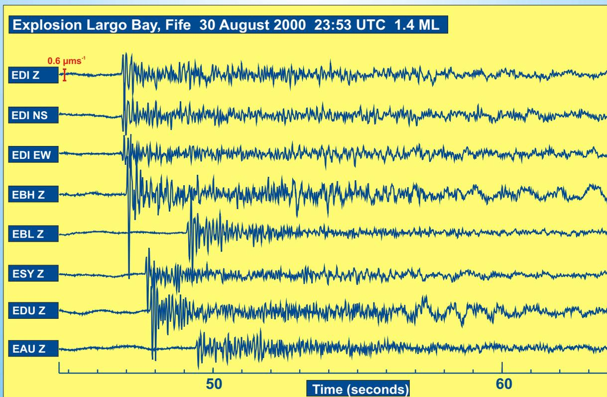
**Figure 20.** Seismograms recorded on the LOWNET (Edinburgh) network from the magnitude 1.4 ML explosion felt in the Leven area on 30 August 2000 23:53 UTC. Three letter codes refer to stations in Annex E.
