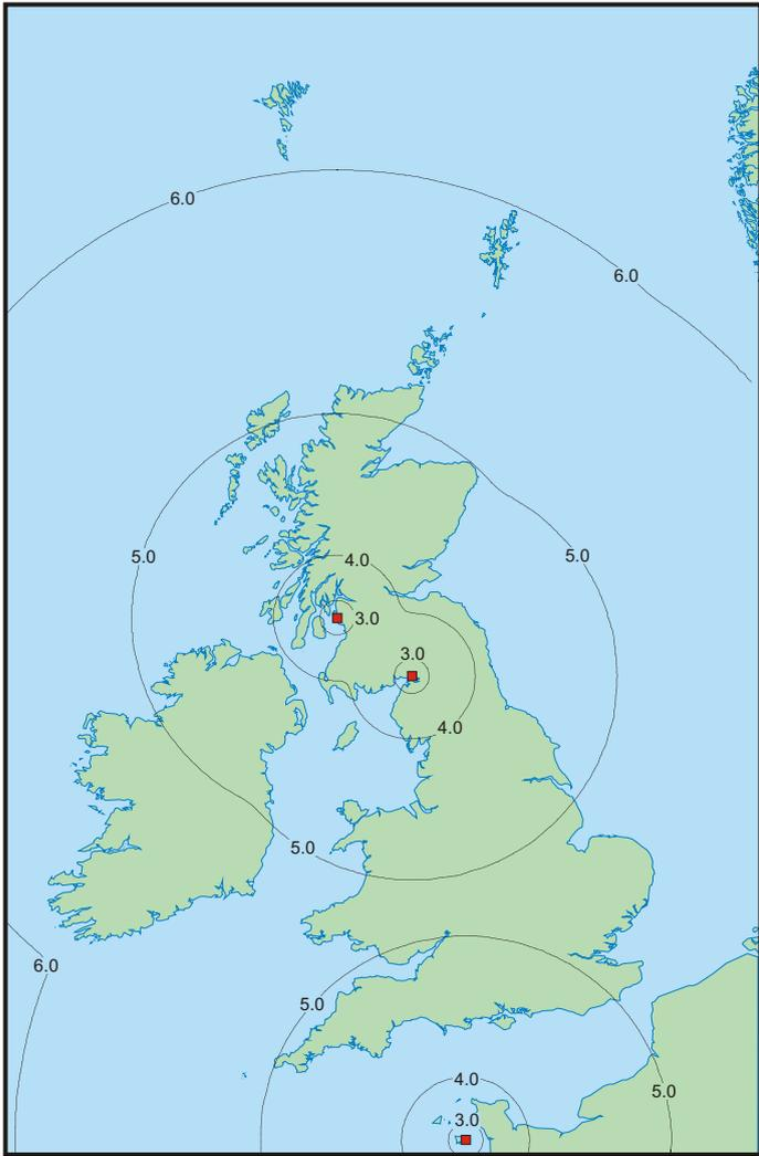
**Figure 7.** Minimum Richter local magnitude (ML) detectable by the strong motion network operational December 1992.
