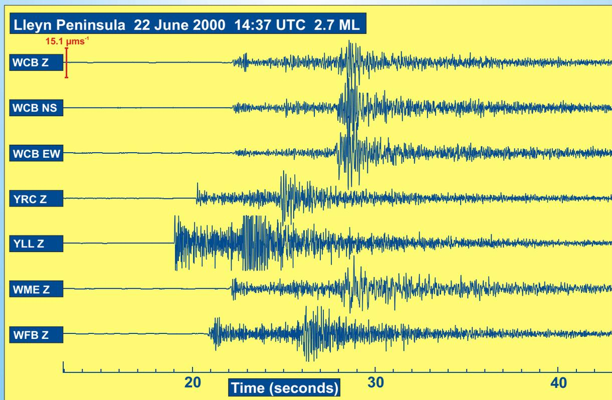
**Figure 14.** Seismograms recorded on the North Wales network from the magnitude 2.7 ML earthquake felt in the Gwynedd area on 22 June 2000 14:37 UTC. Three letter codes refer to stations in Annex E.
