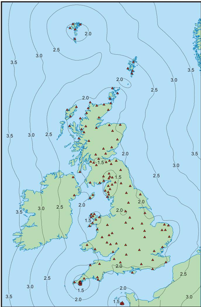
**Figure 3.** Detection capability of network, March 2001. Contour values are Richter local magnitude (ML) for 20 nanometres of noise and S-wave amplitude twice that at the fifth nearest station.
